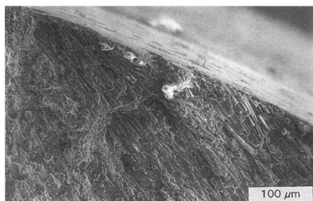
Figure 10 Fracture origin of a composite tensile specimen.
